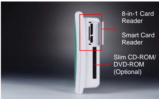
Picture 2.3: Left view of the Medical Station
