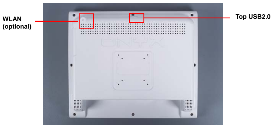
Picture 2.2: Rear view of the Medical Station
