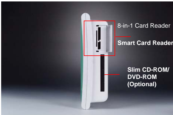
Picture 2.3: Left view of the Medical Station
